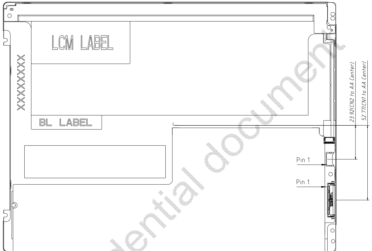
Figure 17 Reference Outline Drawing (Back Side)
